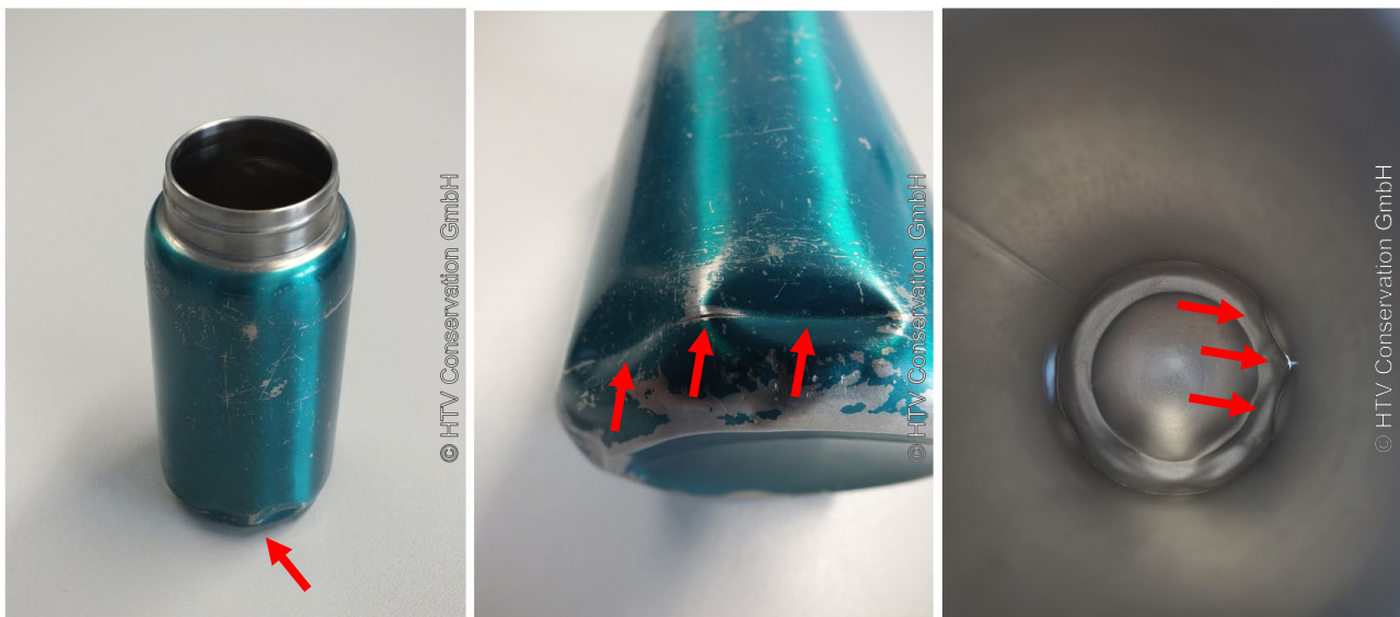
Abbildung 1: Defective product after mechanical impact (damage area, red)
