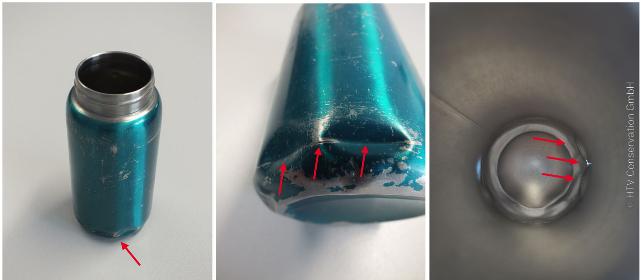
Figure 1: Defective product after mechanical impact (damage area, red)
